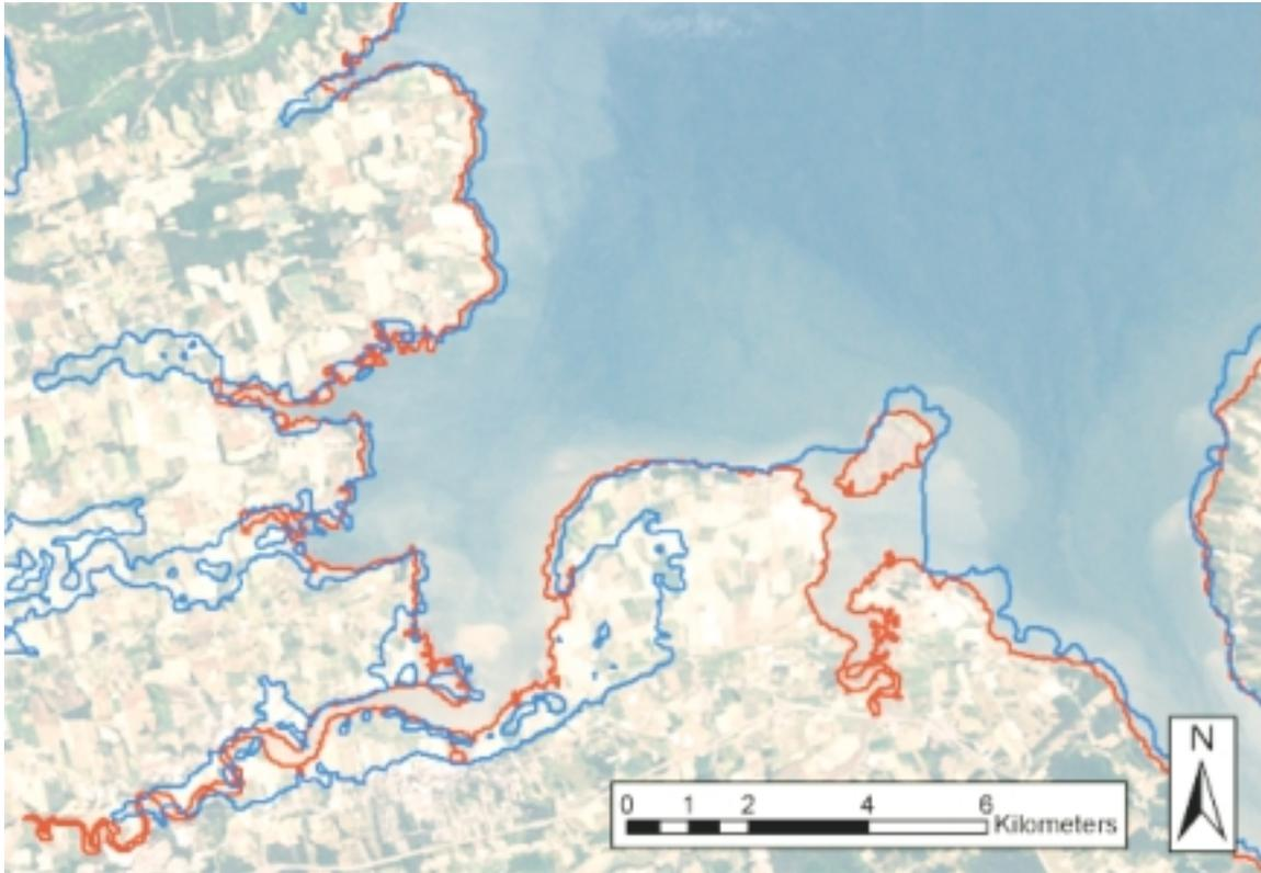
Fig. 9 True colour Landsat-7 image of the Wolfville vicinity at 14:52:00 (GMT) on 13 July 2000. The image was taken near high tide. The red line is the instantaneous coastline extracted from one of the near infra-red bands and the blue line is the coastline extracted from the tidal model. The analysis is reported in Milne (2003). Image courtesy of Trevor Milne and the Applied Geomatics Research Group.
